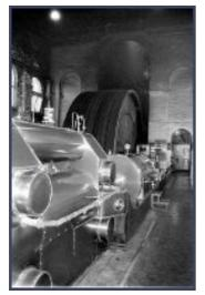
Blackburn. the flywheel was increased in size from 43 grooves for 1.5/8" (41mm) ropes to 44 grooves to accept ropes of 1.7/8" (47.6mm) diameter. 58.5 revolutions per minute, the new engine could produce 2650 IHP (indicated horse power).
